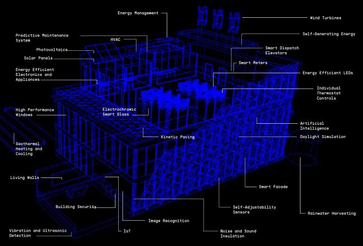
A Digital Twin generally consists of a 3D graphic of the structural components of the building (think of a BIM model illustrating the building's outline, its walls, floor plans, internal systems). This graphic then incorporates all of the devices and sensors within a building to showcase all of the past and present data, ultimately creating a real-time picture of what is happening in the building at that precise moment.
